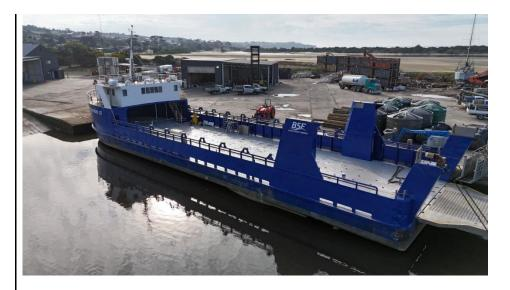
Above; Deck yards and stock boxes removed ready for a general freight run to Flinders Island. It takes about 2 hours to reconfigure the vessels. Below: Freight under the stock boxes with yards stowed, containers on the stern on the way to the Island to pick up a full load of livestock once the yards have been set up. Cattle walk onto the vessel via the stern ramp and a loading race up to the stock boxes.
