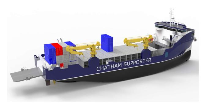
The cargo hold of the proposed vessel has a total internal volume of approximately **2,820 m<sup>3</sup>**, with dimensions of **5.800 m** high, **13.900 m wide**, and **35.000 m long**.
